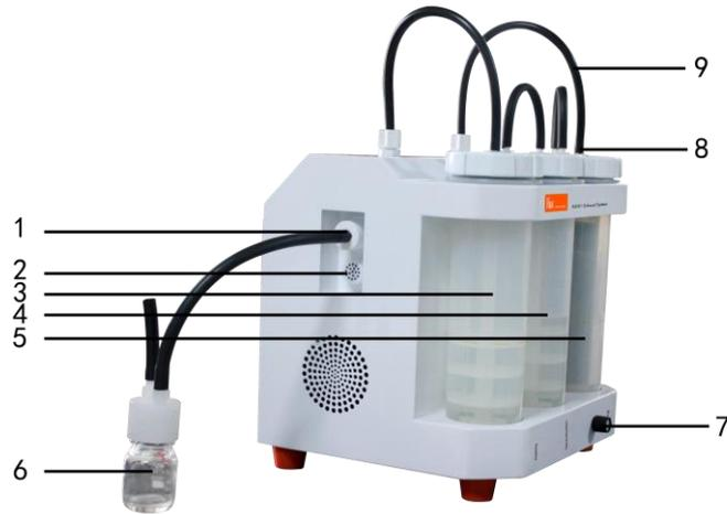
1. Air inlet 2. Air outlet 3. Washing tank 4. Neutralization tank 5. Drying tank
