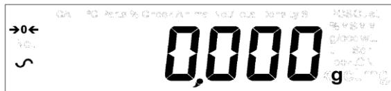
The display will show zero reading along with the zero symbol “ $\rightarrow 0 \leftarrow$ ” and the weighing unit last used. If automatic time calibration is enabled the balance will calibrate 15 minutes after power up, or again after the pre-set time interval.
